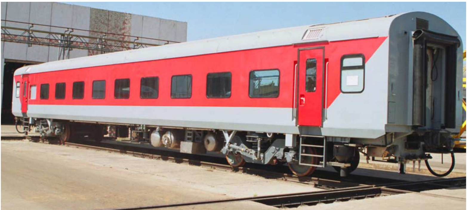
Figure 6 : LHB coach used on Rajdhani Express. This image is taken from Reference [15].
